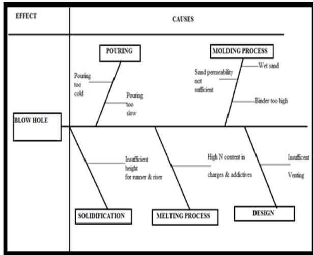
**Figure.5** Cause & Effect Diagram
