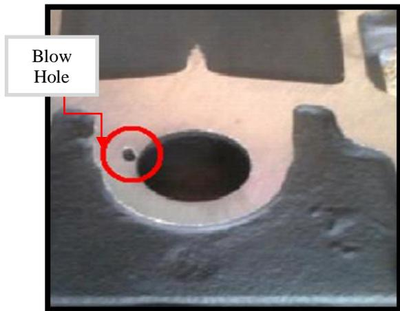
**Figure.8** Blow Hole Due To Core
