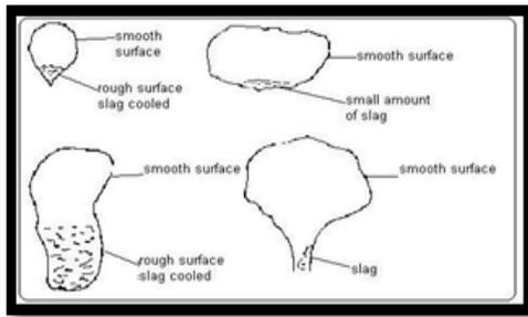
**Figure 2** Slag Blowholes [7]
