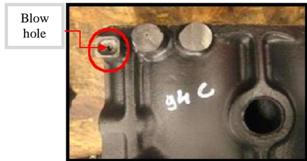
**Figure.6** Blow Hole on Face of Component
