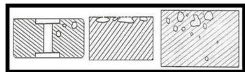
Figure.1 Schematic of Blow Holes [7]
