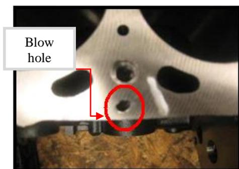
**Figure.10** Blow Hole on Head Face
