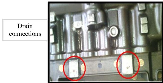
**Figure.11** Drain Connection Provided
