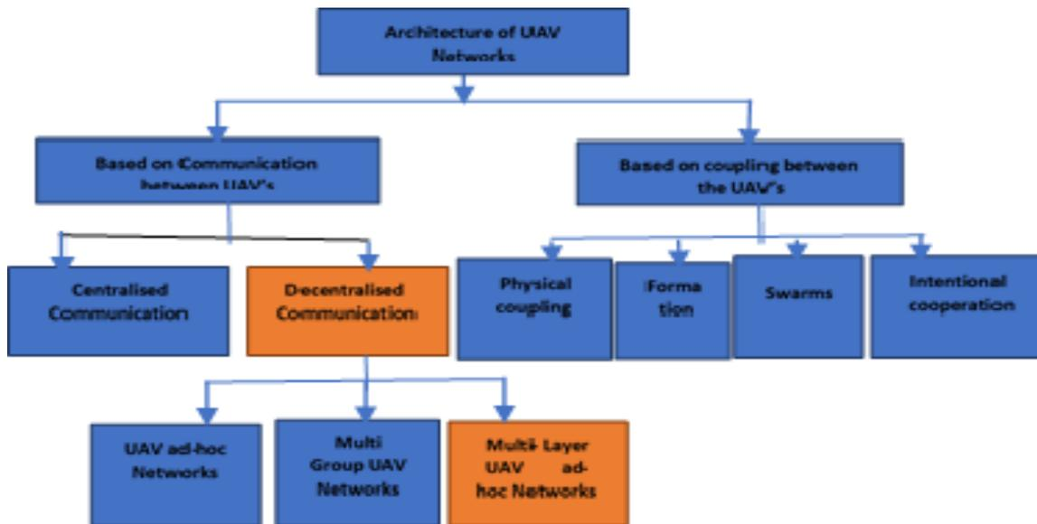
Fig.1. Classification of Architecture of UAV networks.
