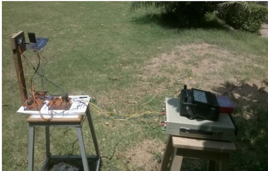
**Fig. 2:** Designed working Prototype of solar tracker.
