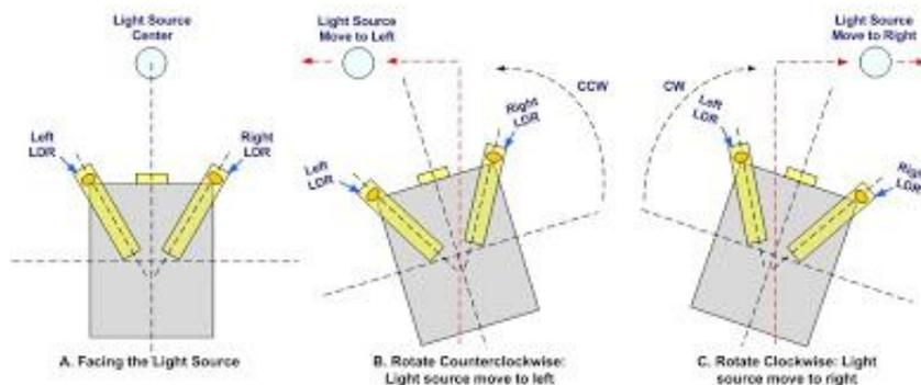
**Fig. 1:** Concept of using two LDRs for sensing.
