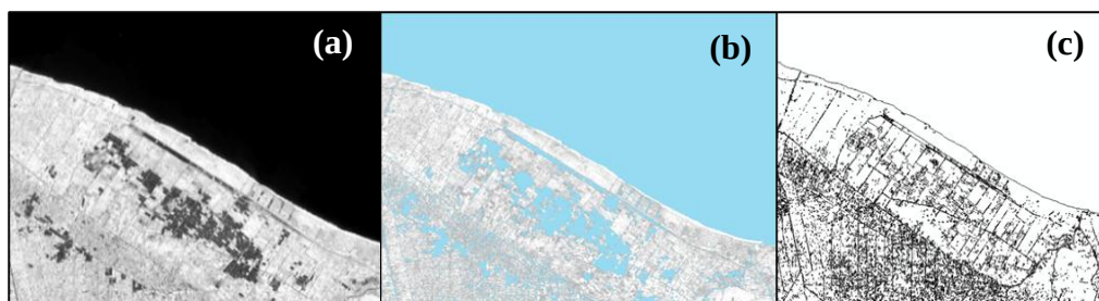
Figure. 4 The methodology for shoreline extraction in 2022 includes; a Landsat raster image of Band 5; b the binary image; c the vector map (polygon shapefile).
