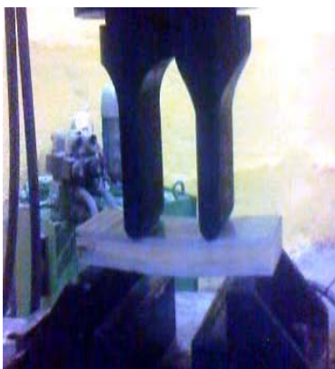
Fig 3: Quarter point loading test
