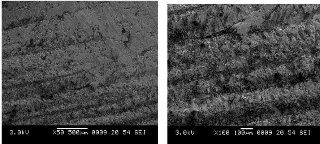
**Figure 6:** SEM micrograph of the worn surface of specimen C3 with 50x & 100x magnification
