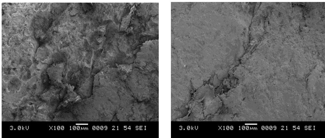
**Figure 7:** SEM micrograph of the worn surface of specimen C4 with 100x magnification.
