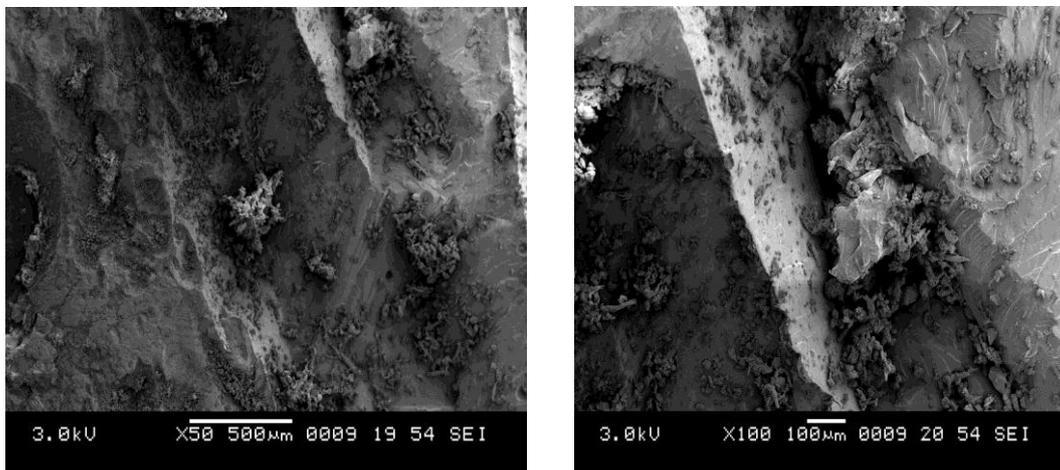
**Figure 5:** SEM micrograph of the worn surface of specimen C2 with 50x &100x magnification.
