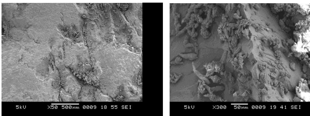
**Figure 4:** SEM micrograph of the worn surface of specimen C1 with 50x & 300x magnification.
