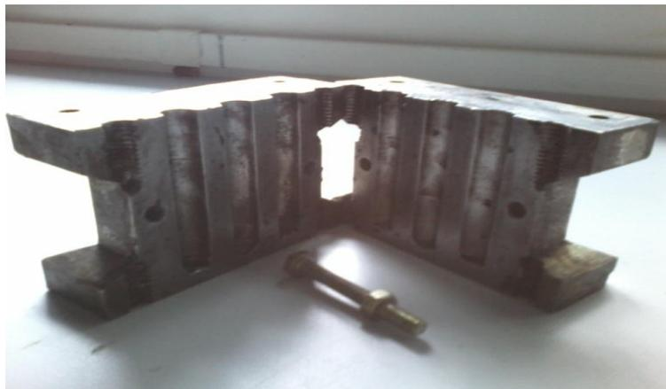
**Figure1:** Metallic die For Preparation of Specimen.
