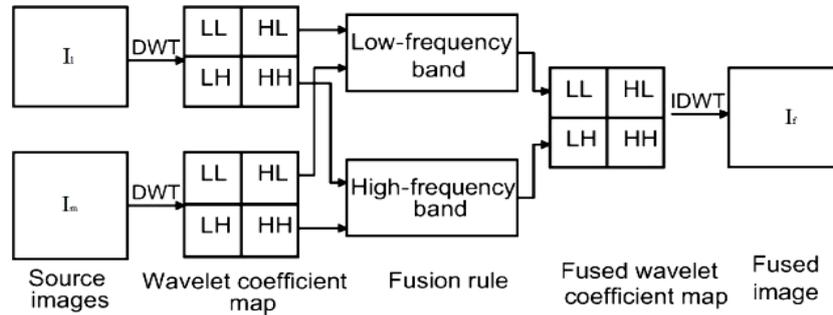
**Figure 2:** Flow chart of DWT based Image Fusion [8]
