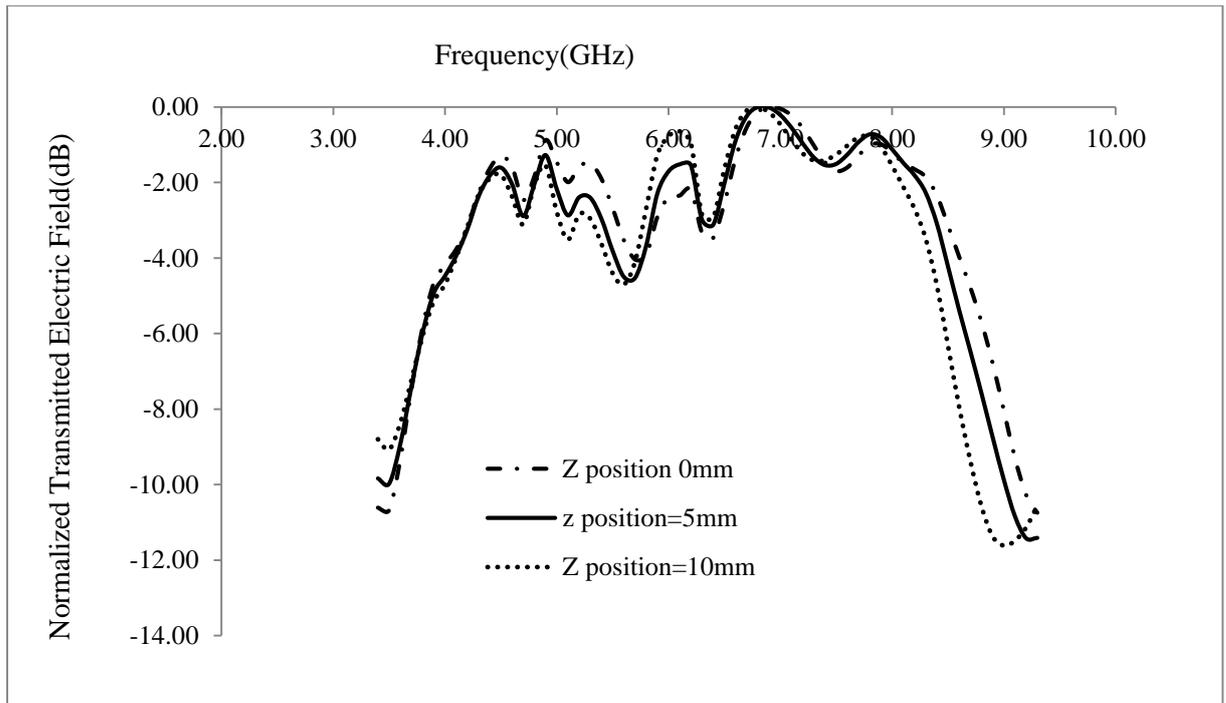
**Figure 6:** Transmission characteristics of FSS at various distance between receiving horn antenna and curved FSS along Z -axis
