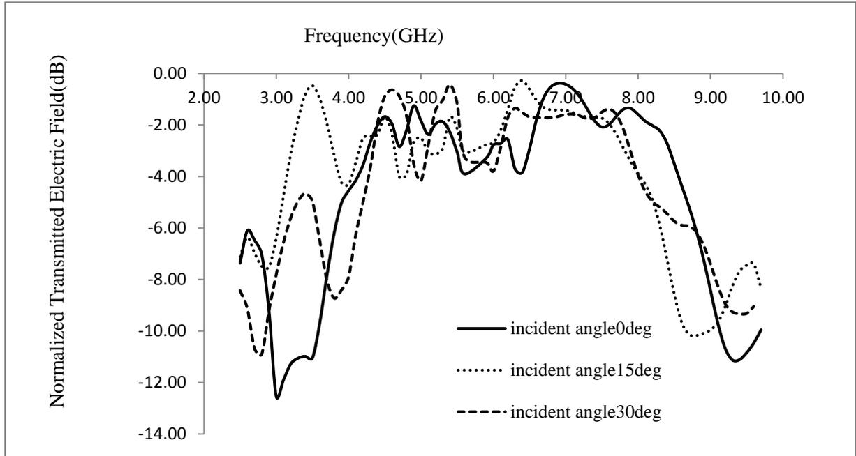
**Figure 5:** Transmission characteristics of FSS at various incident angles
