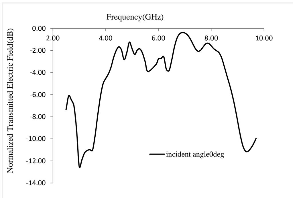
**Figure 4:** Transmission characteristics of FSS at 0 degree incident angle
