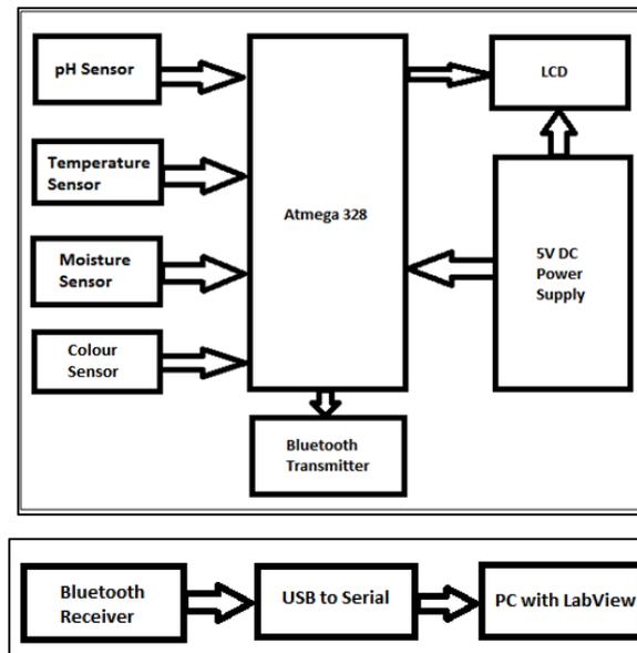
**Figure 1:** Block diagram of water quality monitoring system.
