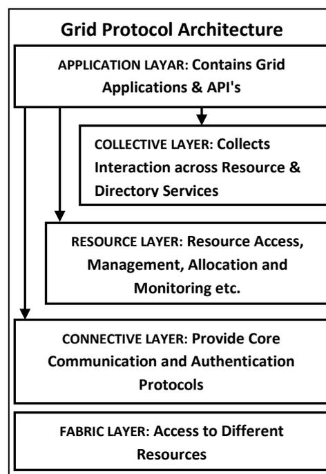
**Figure 8.** Layered Architecture of Grid System reproduced from [21], [71]
