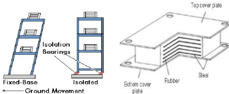
**Fig. 1:** Behavior of Fixed base & isolated base buildings.
