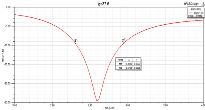
Fig 5: The simulated Returnloss of the designed 5G mobile antenna at solution frequency of 3.5 GHz where length of ground (Lg=37.6)
