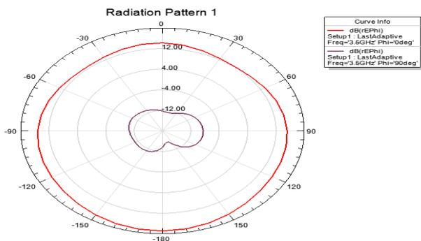
Fig 11: The simulated near field pattern of the proposed antenna at 3.5 GHz
