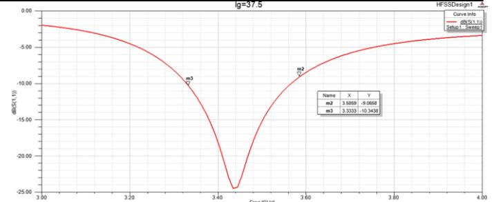
Fig 4: The simulated Returnloss of the designed 5G mobile antenna at solution frequency of 3.5 GHz where length of ground (Lg=37.5)
