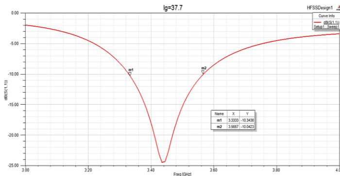
Fig 6: The simulated Returnloss of the designed 5G mobile antenna at solution frequency of 3.5 GHz where length of ground (Lg=37.7)
