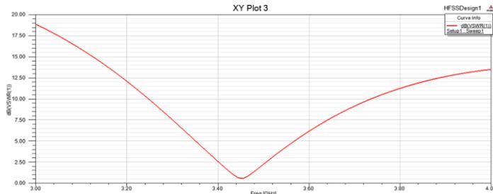
Fig 9: The simulated VSWR of the designed 5G mobile antenna at solution frequency of 3.5 GHz
