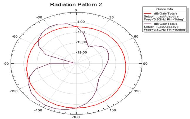
Fig 12: The simulated far field pattern of the proposed antenna at 3.5 GHz
