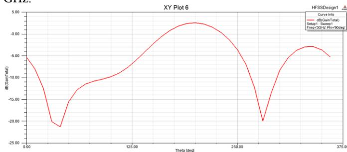
Fig 10: The simulated Gain of the designed 5G mobile antenna at solution frequency of 3.5 GHz
