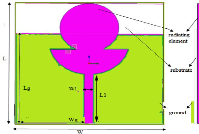
Fig 3: Proposed geometry of Antenna configuration.
