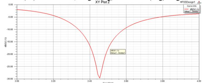
Fig 8: The simulated Returnloss of the designed 5G mobile antenna at solution frequency of 3.5 GHz
