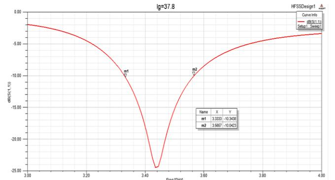
Fig 7: The simulated Returnloss of the designed 5G mobile antenna at solution frequency of 3.5 GHz where length of ground (Lg=37.8)
