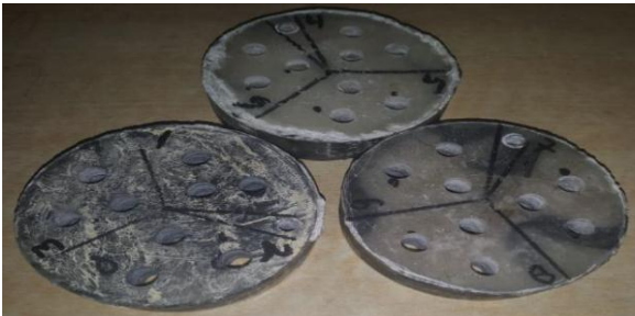
Figure2: Drilled compression molded carbon filled GFRP specimen
