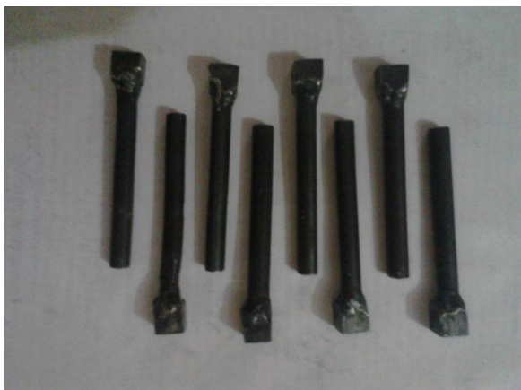
Figure 1: Specimen for wear test
