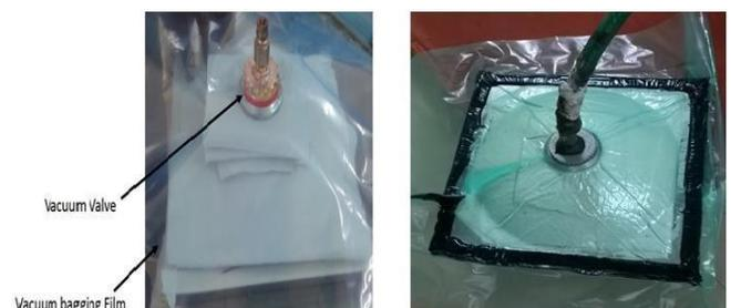
Figure 3: Vacuum bagging and air suction process
