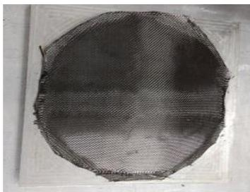
**Figure 4:** Layers of carbon fibers
