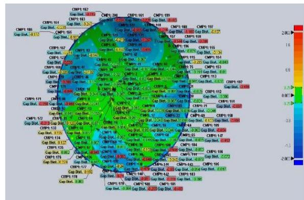
**Figure 8:** Deviation contour plot for composite reflector
