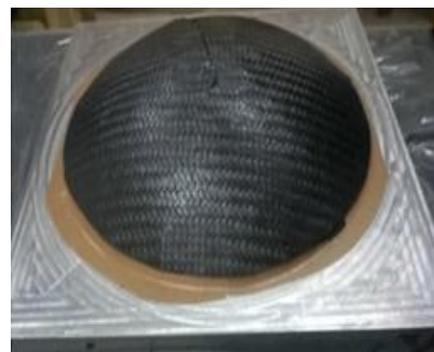
Figure 2: Layers of CFRP prepreg on steel mould
