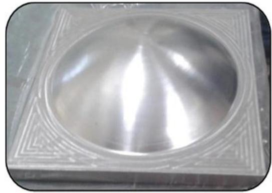
Figure 1: Manufactured stainless steel mould
