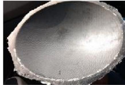
**Figure 7:** Cured reflector manufactured using VARTM process
