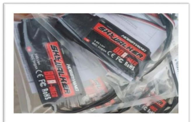
Figure 3.2 Electronic Speed Controller
