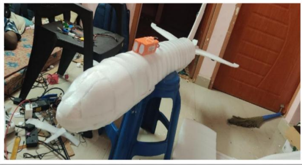
Figure 4.4 Fuselage setup with T-Tail configuration
