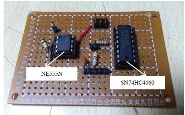
**Fig 7:** Astable oscillator and signal conditioning hardware
