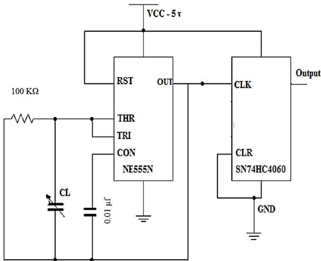
**Fig 6:** Astable oscillator and signal conditioning circuit
