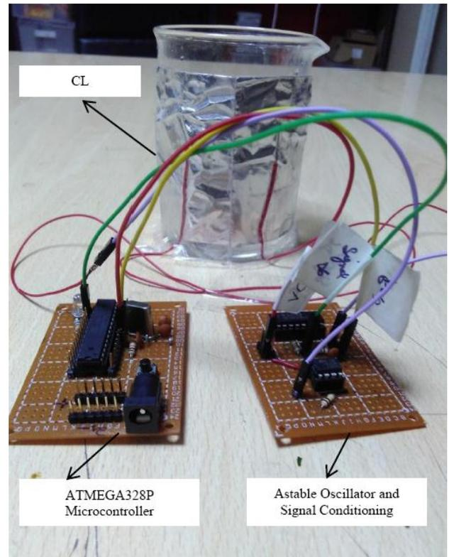
**Fig 8:** Prototype implementation.
