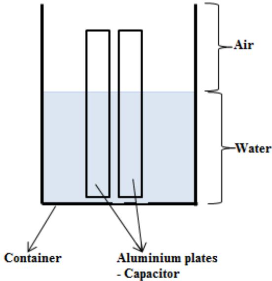
**Fig 2:** Aluminium plate capacitor placed on the surface of glass container
