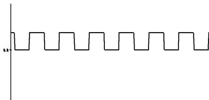
Fig 10: Captured signal with 100 ml of water inside the container
