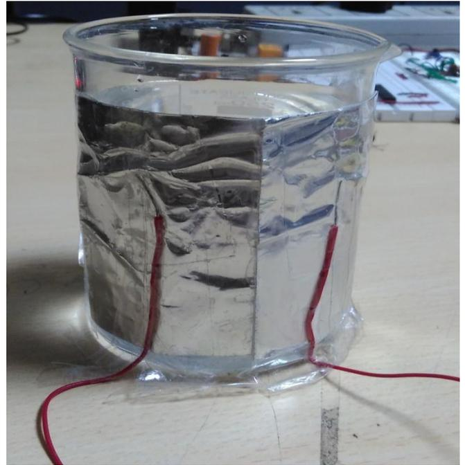
**Fig 4:** Aluminium plate capacitor on glass container
