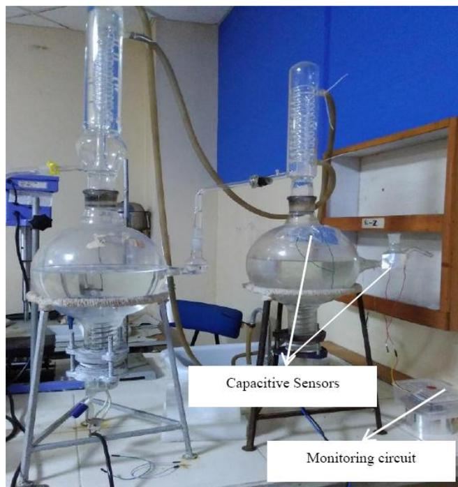
Fig 1: Double distillation plant.
