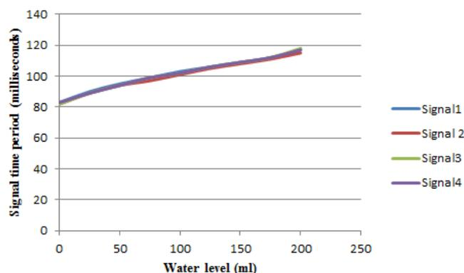
Fig 11: Change in signal time period with change in water level.
