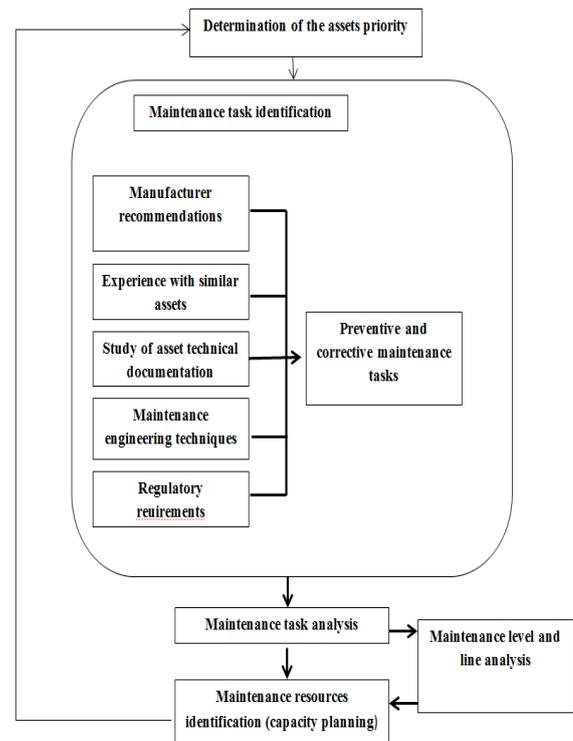
Figure 5: Maintenance task and capacity planning model
