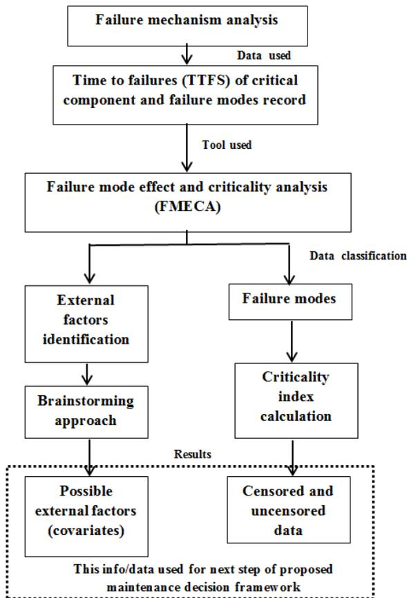
**Figure 3:** The process of failure mechanism analysis
