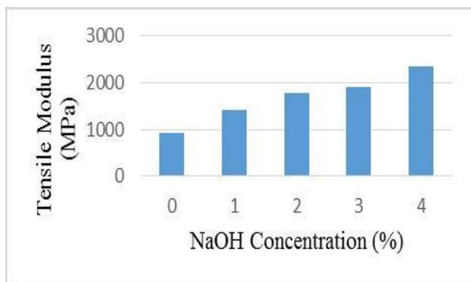
**Figure 3.** Tensile modulus of untreated and alkali treated Bamboo fiber reinforced epoxy composites.
