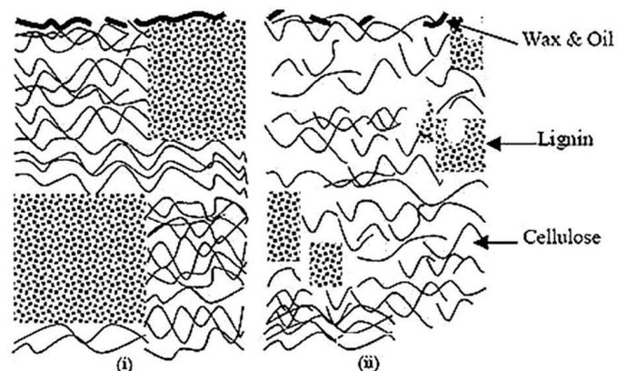
**Figure 1.** Typical structure of (i) untreated and (ii) NaOH treated natural fiber
