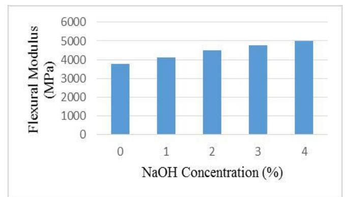
**Figure 5.** Flexural modulus of untreated and alkali treated Bamboo fiber reinforced epoxy composites.
