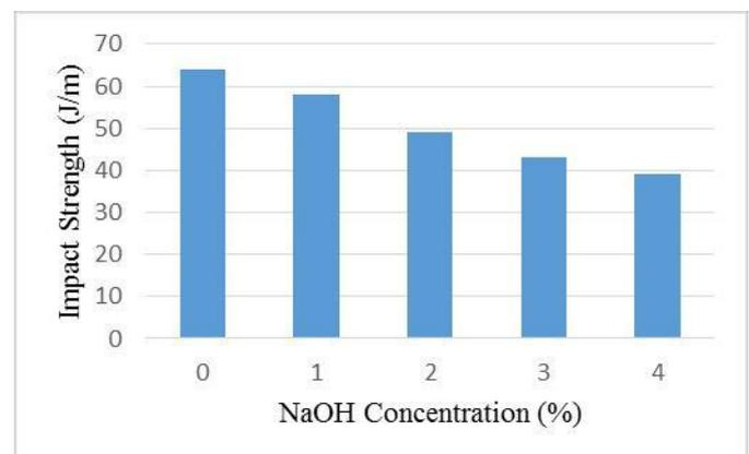
**Figure 6.** Impact strength of untreated and alkali treated Bamboo fiber reinforced epoxy composites.
