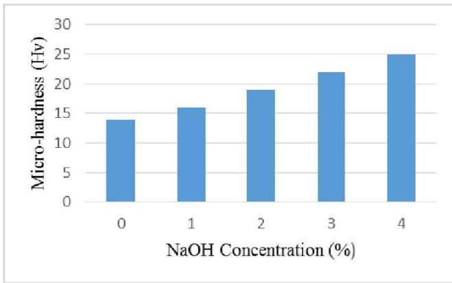
**Figure 7.** Micro-hardness of untreated and alkali treated Bamboo fiber reinforced epoxy composites.
