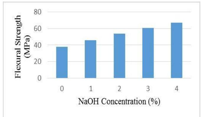
**Figure 4.** Flexural strength of untreated and alkali treated Bamboo fiber reinforced epoxy composites.
