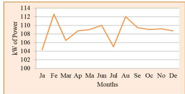
Figure 10: Power output obtained from wind for one year at 26m elevation
