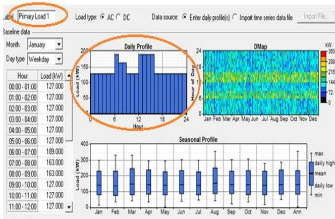
Figure 5: Load Input Window of HOMER by Taking Primary Load 1 as Sample
