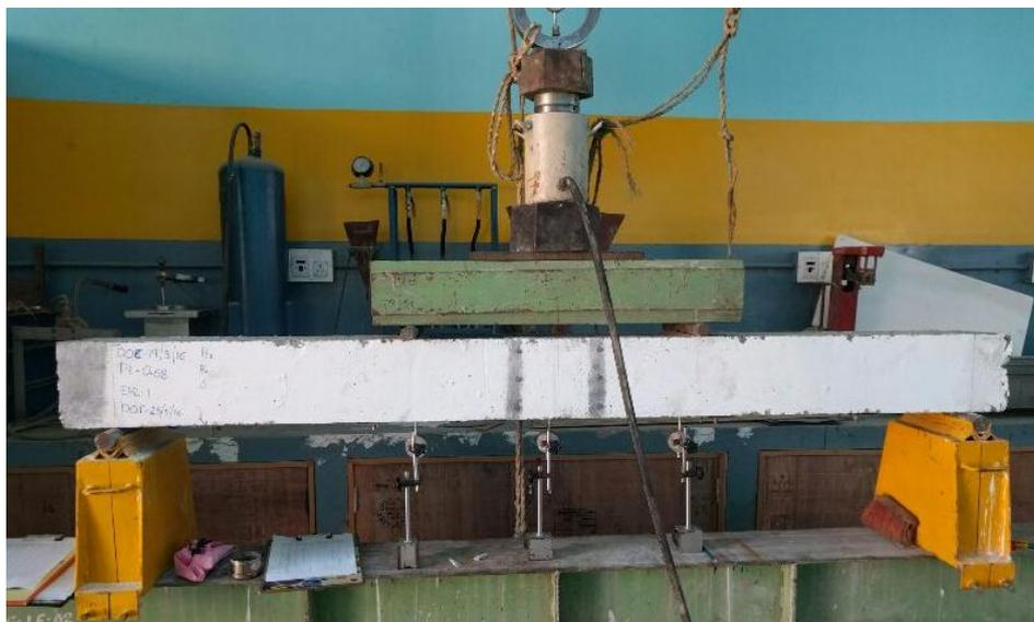
**Figure 3.** Experimental Setup for two point loading
