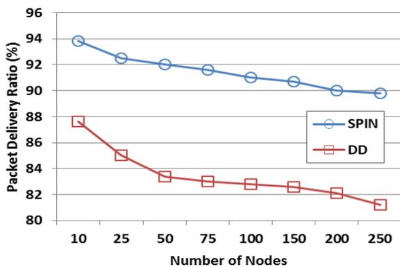
**Figure 1** Packet Delivery Ratio at Random Waypoint Mobility Model
