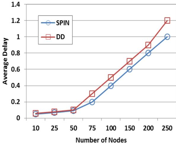
**Figure 3** End-to-End Delay at Random Waypoint Mobility Model
