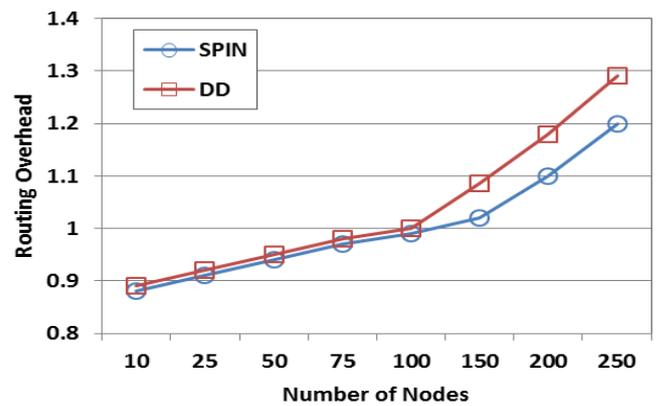
**Figure 2** Routing Overhead at Random Waypoint Mobility Model
