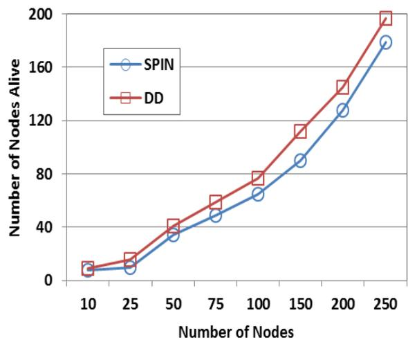
Figure 12 Network Lifetime at RPGM Mobility Model
