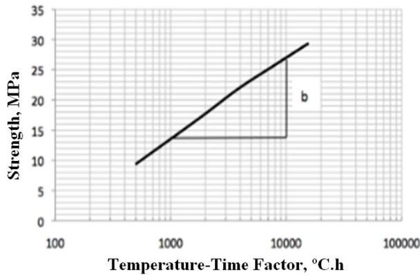
Figure 1. Cumulative temperature-time vs concrete strength
