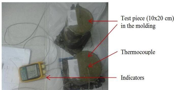
**Figure 2.** Equipment for temperature recording
