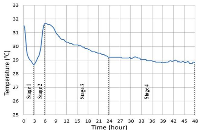
**Figure 3.** Temperature of the concrete in four stages
