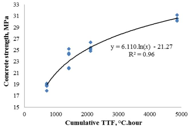
**Figure 4.** The cumulative-TTF vs concrete strength
