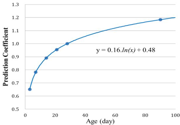
**Figure 6.** Prediction coefficient vs concrete age
