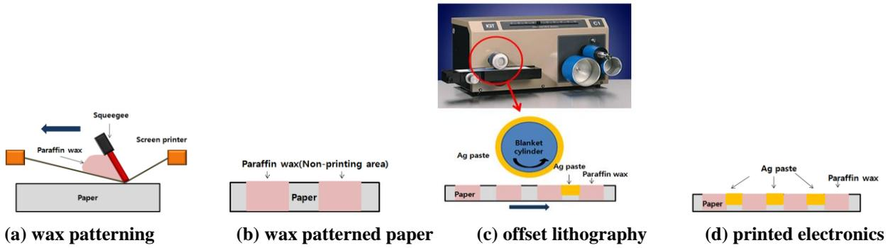
**Figure 1.** Schematic diagram of WPOP (wax patterning offset printing) process for the manufacturing a printed electronics.
