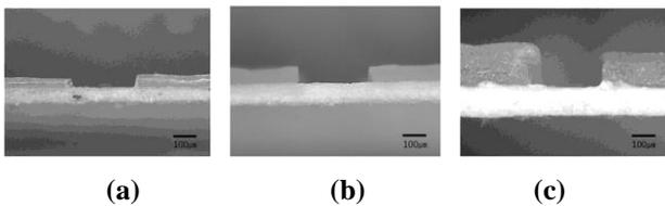
**Figure 2.** Cross sectional view of wax printed papers by screen printing. (a), (b) and (c) are samples of 1, 2 and 3 respectively.
