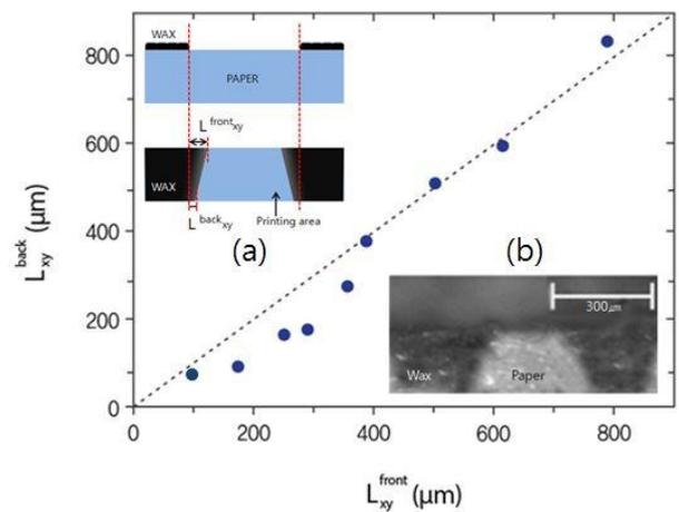
**Figure 3.** Cross sectional view of paper sample which was patterned by wax. Schematic (a) is a wax patterned model and photography (b) is a wax patterned paper sample 1.
