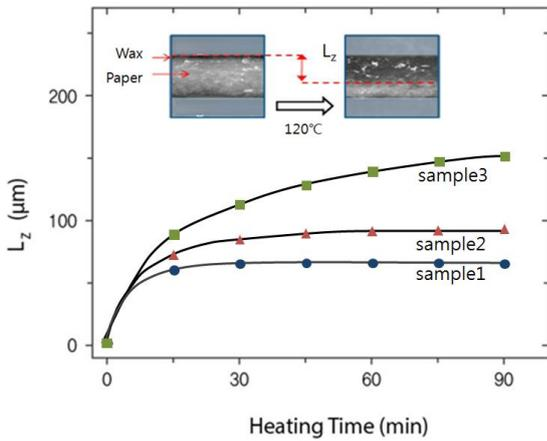
**Figure 4.** Microscopic measurements of depth of penetration of wax pattern onto papers. (a),(b) and (c) are the sample of 1, 2, and 3 respectively.
