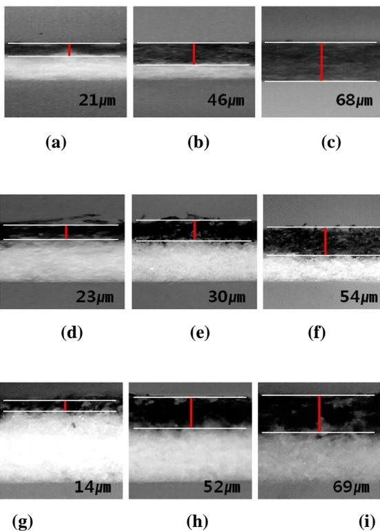
**Photograph 1.** Cross sectional views and depth of penetration of inks onto paper samples. ((a)~(c) are sample of 1, (d)~(f) are sample of 2, and (g)~(i) are sample of 3.) (a),(d) and (g) were printed under 100N, and (b),(e) and (h) were printed under 300N, and (c),(f) and (i) were printed under 500N printing pressure by WPOP method respectively..
