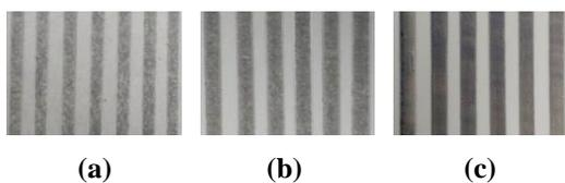
**Figure 5.** Printed patterns of conductive ink on papers printed by WPOP method. (a), (b) and (c) are sample of 1, 2 and 3 respectively. The width of a line of each pattern is 100 µm.
