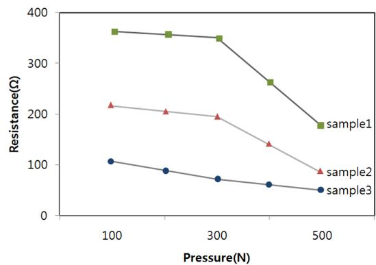
**Figure 6.** Electric resistances differences on the depth of conductive silver paste inks at temperature 80°C.
