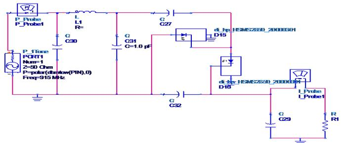
**Figure 3:** Single stage voltage doubler RF energy harvesting circuit with  $\pi$  type matching network
