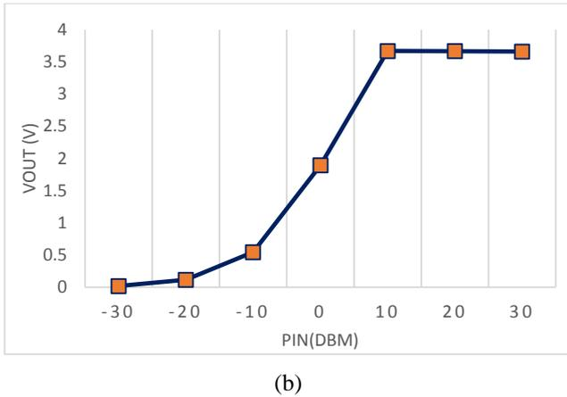
**Figure 4:** Output voltage for  $\pi$  type matching circuit for single stage (a) input-output voltage as function of time (b) Output voltage vs PIN(input power dBm)
