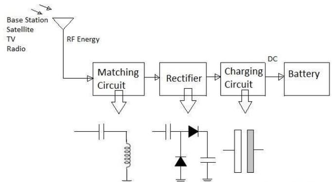
**Figure 1:** Typical block diagram of RF energy harvesting circuit
