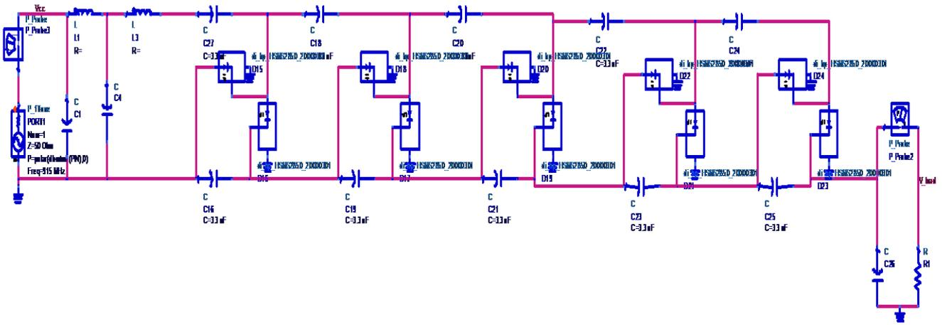
**Figure 5:** RF harvesting circuit design using 5 stage voltage multiplier with diode HSMS-2850 (Agilent ADS)
