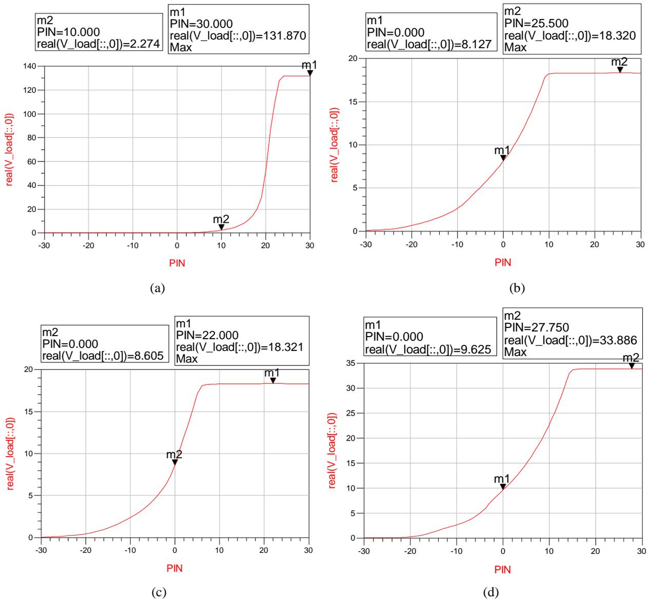
**Figure 6:** Output voltage of five stage RF harvesting circuit for different diodes (a) Diode-HSMS-2822 (b) HSMS-2850 (c) HSMS-2852 (d) HSMS-2860 (PIN = Input Power)
