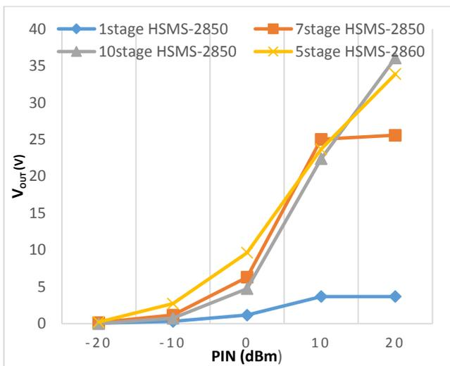
**Figure 7:** Output voltage of 1, 7, 10 and 5 stages RF harvesting circuit for diode HSMS-2850 and HSMS-2860 respectively
