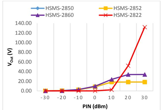
**Figure 8:** Output voltage of 5 stage RF harvesting circuit for diode HSMS-2822, HSMS-2850, HSMS-2852 and HSMS-2860
