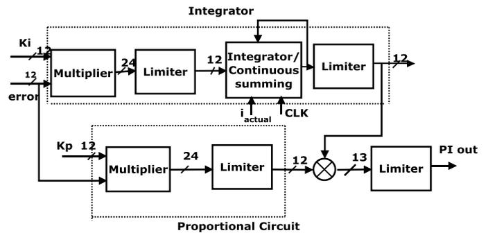
Figure 11. Logical Implementation of PI Controller with FPGA
