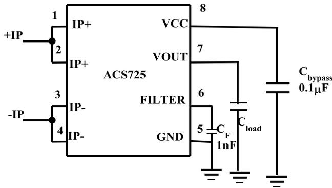
Figure 5. Circuit Arrangement of ACS 725
