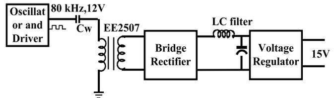
Figure 4. Isolated power Supply for Driver Circuit
