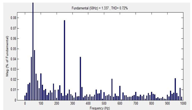
Figure 16. Fourier analysis of grid current waveform
