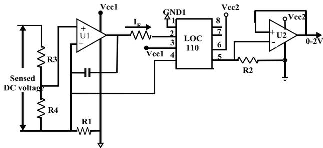
Figure 6. Configuration of LOC 110 for DC bus voltage sensing
