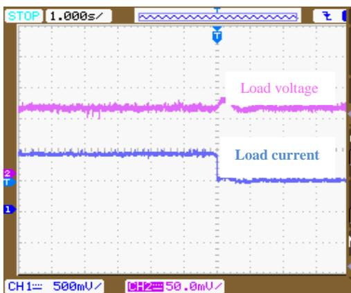
**Figure 18.** Response of dc link voltage for a load change.
