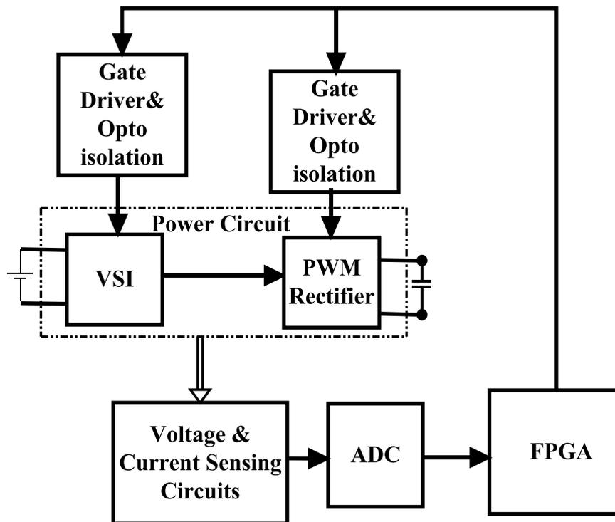
Figure 1. Functional Blocks of Experimental Setup
