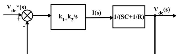
Figure 9. PI controller for dc voltage regulation
