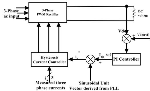
Figure 8. Controller for PWM Rectifier
