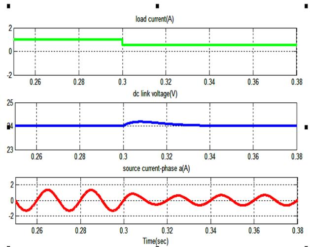
Figure 14. Dynamic response of DC output voltage and source current
