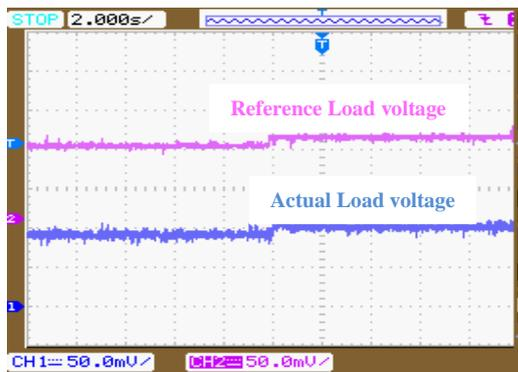
**Figure 17.** Response of dc link voltage for a reference change.
