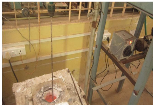
Fig. 1 Stir casting setup
