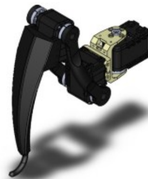
Fig 6. CAD design of the paw of the hexapod robot.
