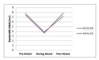
**Figure 4.** Comparison of bandwidth between devices in different scenarios.
