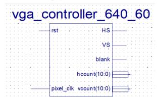
Figure 1: Core that generates system synchronization signals
