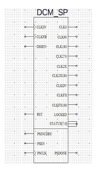
Figure 3: DCM Digital Clock Manager System clock controller
