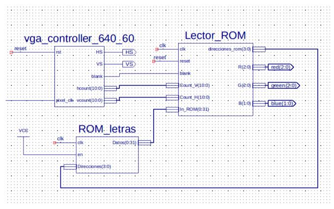
Figure 4: General block diagram of the system
