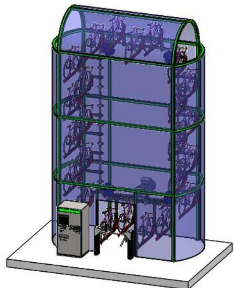
**Figure 14.** Design of vertical rotary parking.
