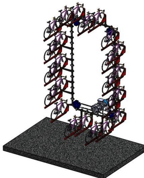
**Figure 4.** Vertical rotating system.
