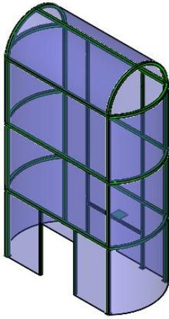
**Figure 9.** Structure and housing of the parking lot.
