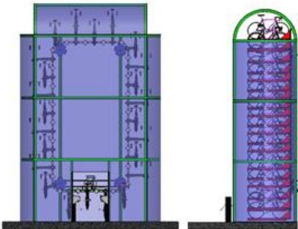
**Figure 10.** Rotary parking design.
