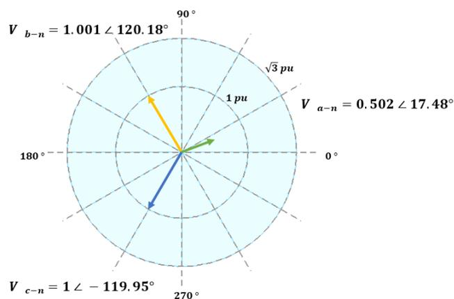
**Figure 7.** Voltage phasors in the PCC – single-phase fault 13-14 directly grounded
