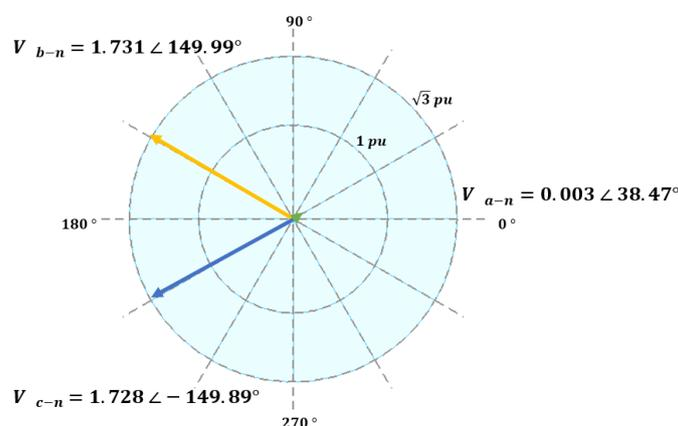
**Figure 9.** Voltage phasor in the PCC- single-phase fault 13-14 with resistive grounding of 88 Ω.
