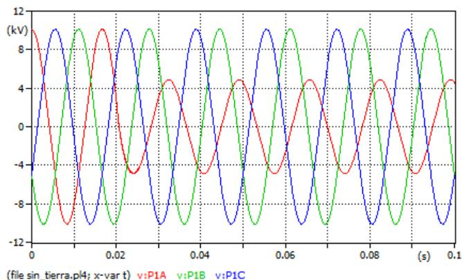
**Figure 6.** Voltages in the PCC before a single-phase failure 13-14 directly grounded.
