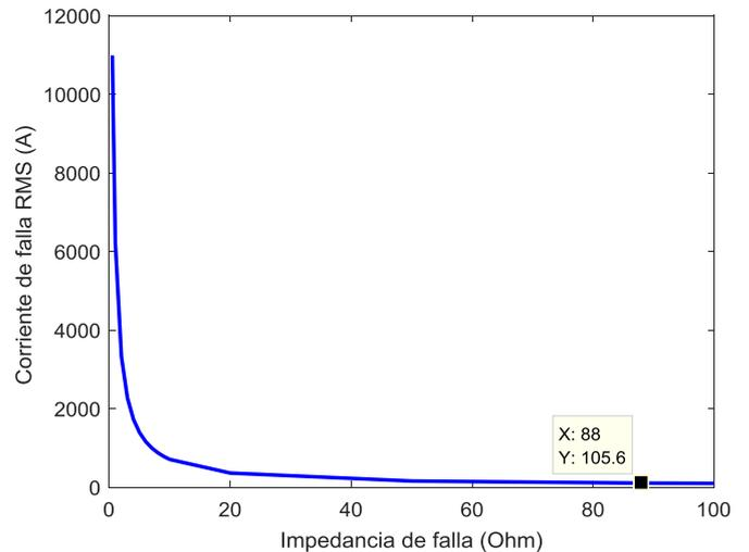
Figure 4. Relation between resistance versus fault current
