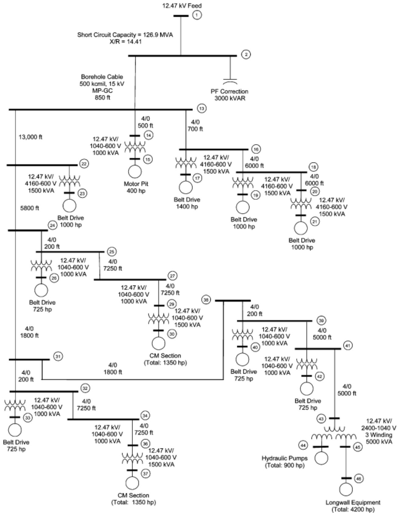
Figure 1. Electrical Power System-Underground Mining [8].
