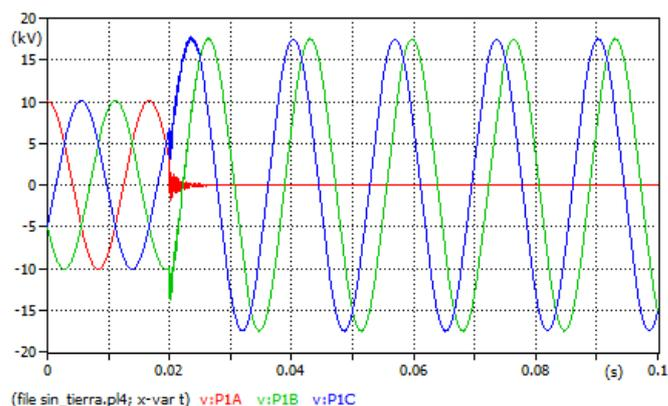
**Figure 8.** Voltages in the PCC before a single-phase fault 13-14 with impedance of resistive grounding of 88 Ω.
