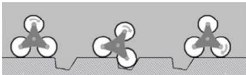
**Figure 2.1:** Tri-Star wheel in motion
