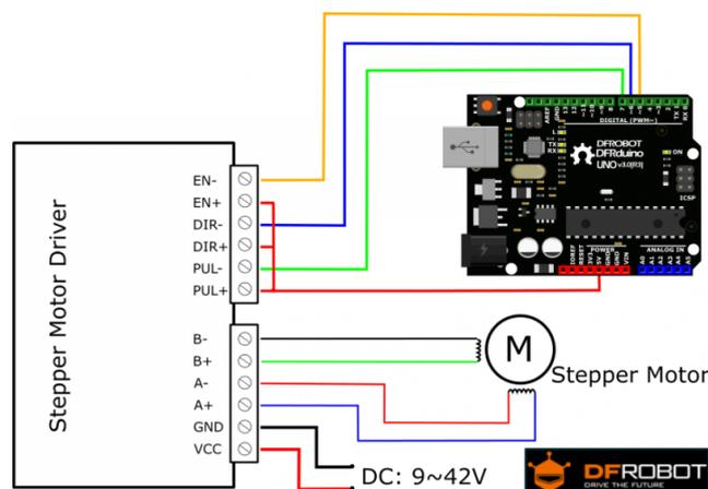
Figure 2.3: Circuit Diagram
