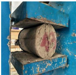
Figure 2.2. Split Tensile Test
