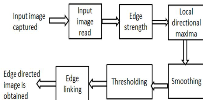
**Figure 1.** Block diagram of Edge detection
