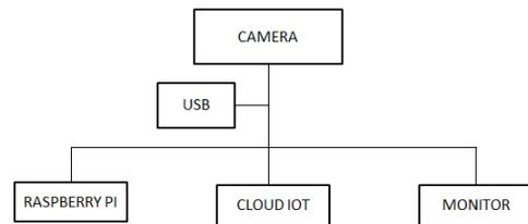
**Figure 4.** Block diagram of the project hardware and software used.
