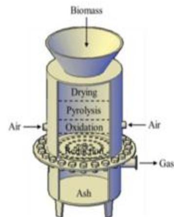
Figure 1. Downstream gasifier [14].
