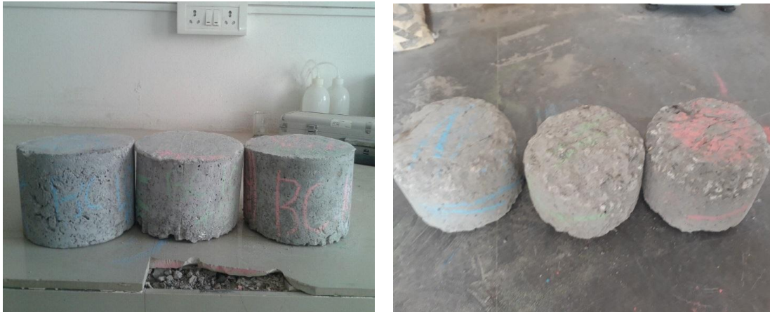
Figure 7. Shape of specimen used in cantabro test at before 50 rev and after 300 rev
