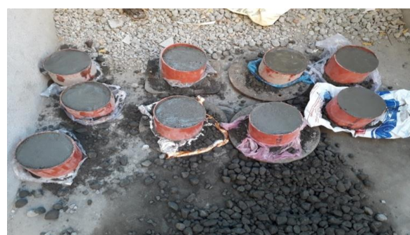
Figure 5. Preparation of samples for cantabro test
