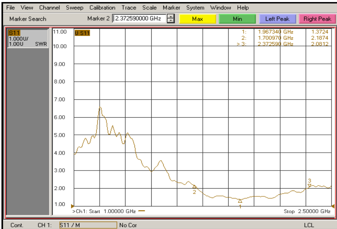
Figure 7. Measured bandwidth of the Antenna resonating at 1.96GHz on Rogers (RT/Duroid5880tm) of Substrate permittivity 2.2. From the plot, it is clear that the value of the Bandwidth obtained is 0.672GHz with a -10dB impedance bandwidth extending between 1.7 GHz to 2.37GHz respectively as indicated by markers 2 and 3.
