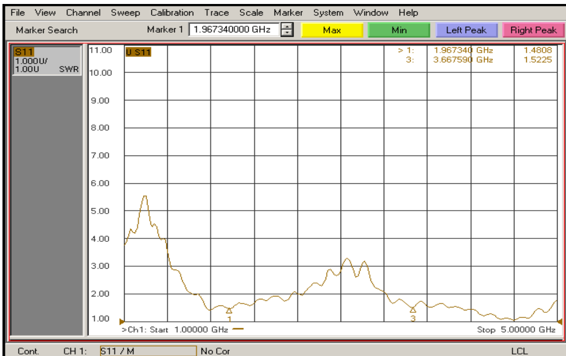
Figure 10. Measured VSWR plot of the Antenna resonating at 1.96 GHz and 3.66GHz indicating a value of 1.48 and 1.52 respectively for the lower and the upper band respectively as indicated by markers 1 and 3 on Rogers(RT/Duroid) substrate of permittivity 2.2.
