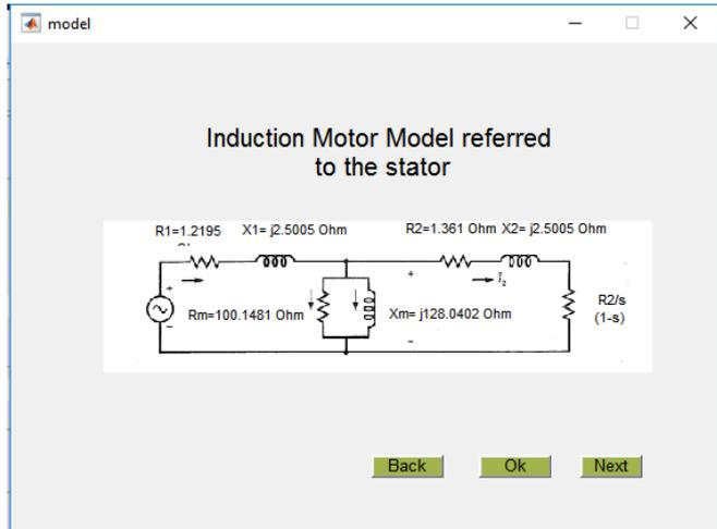
Figure 8: Induction motor model referred to the stator
