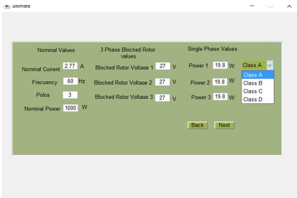
**Figure 4:** Locked rotor test results capture window
