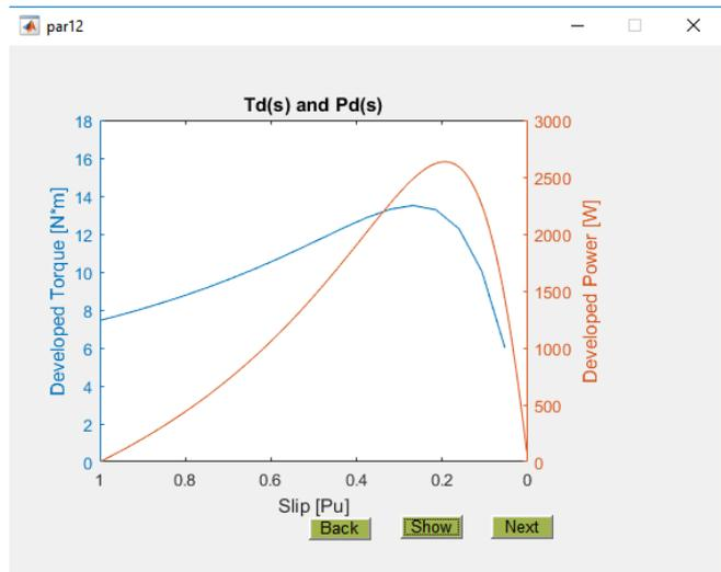
Figure 9: Machine performance curves. Blue curve: torque developed against sliding. Red curve: Power developed against sliding
