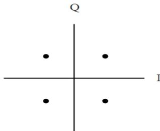
**Figure 2.** Constellation diagram for QPSK modulation.
