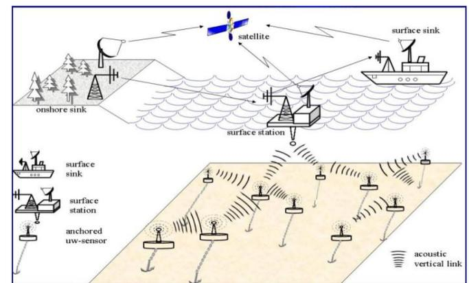
Figure 2. Architecture for 3D Underwater Sensor Network
