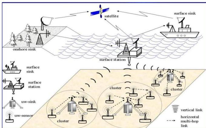
Figure 1. Architecture for 2D Underwater Sensor Networks.
