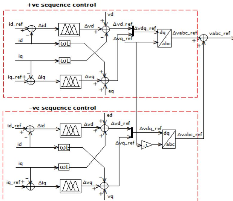
Figure 3. Inner Current control loop with fuzzy logic controller
