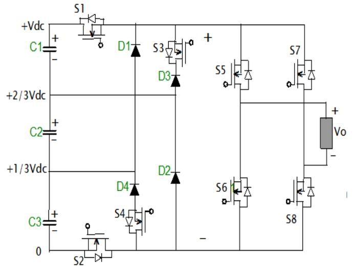
**Figure 4.** Proposed seven-level inverter topology
