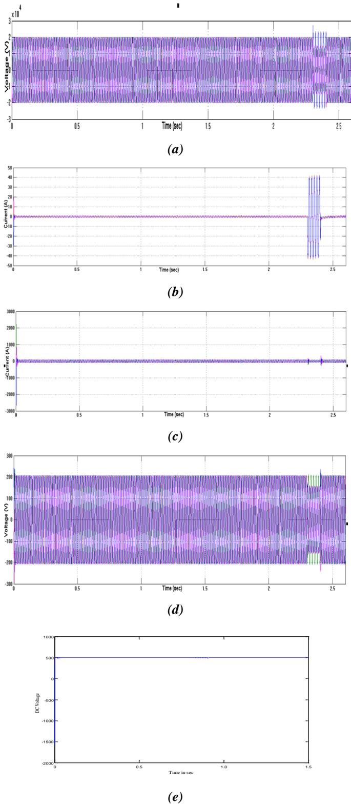
**Figure 5.** Traditional inverter with PR controller under fault (a) voltage at PCC (b) Current at PCC (c) & (d) are the Current and voltage at inverter terminals (e) Inverter input DC link voltage.
