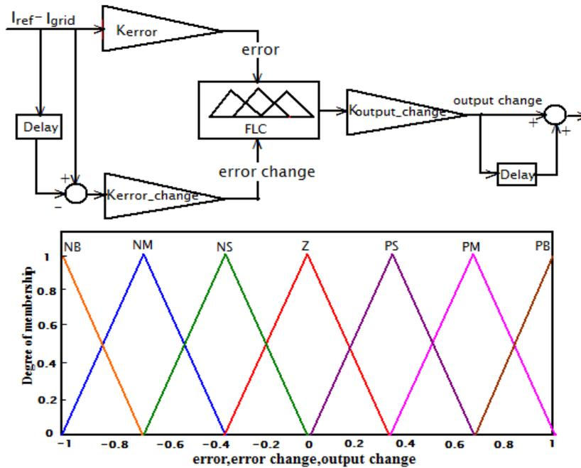
Figure 2.(a) Fuzzy-proportional-integral Controller, (b) Input/output fuzzymembership functions
