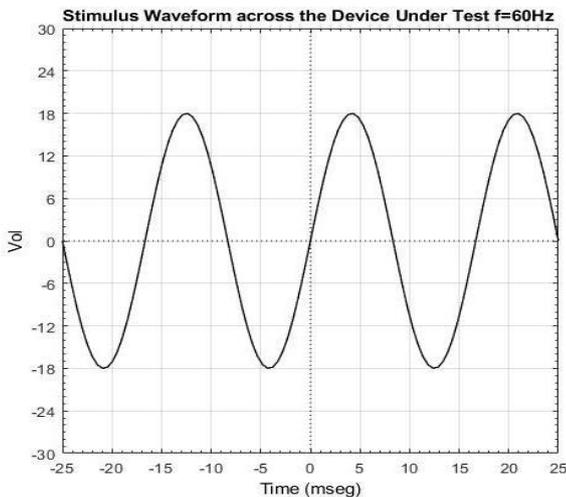
Figure 5. Signal applied to V-I TRACER
