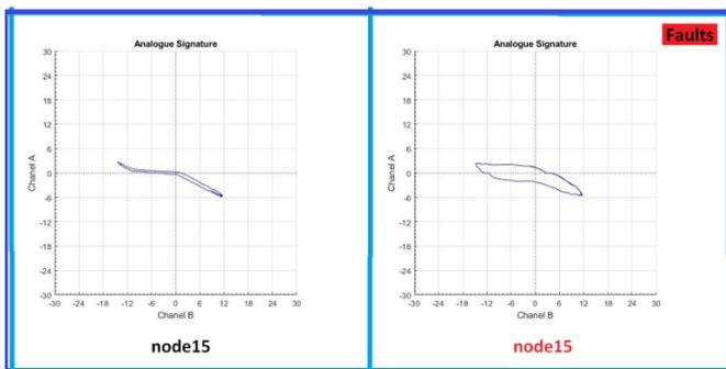
**Figure 8.** Analog signatures on node15 of the cards
