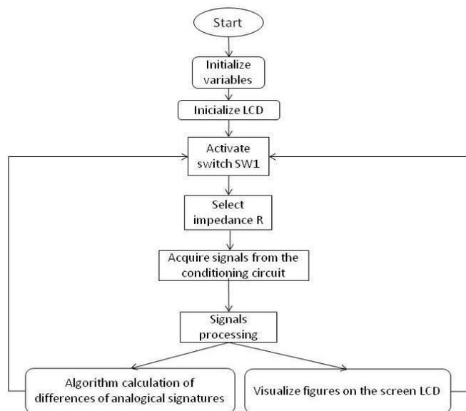
**Figure 2.** Microcontroller algorithm used in the tool
