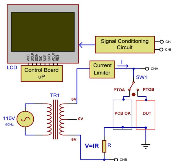
Figure 1. V-I TRACER diagram
