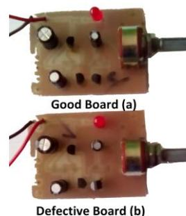
**Figure 3.** Board to diagnose: (a) Good Board, (b) Defective Board
