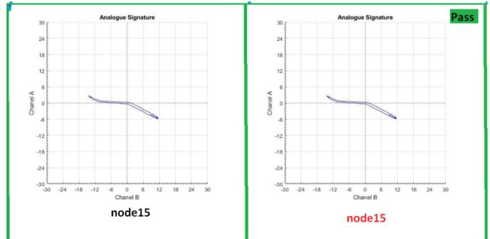
**Figure 10.** Analog signature on node15 of the cards after changing defective components
