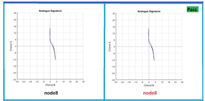
Figure 7. Analog signatures on node8 of the cards
