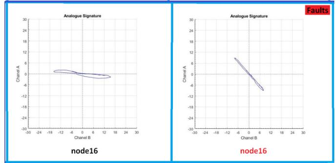
**Figure 9.** Analog signatures on node16 of the cards
