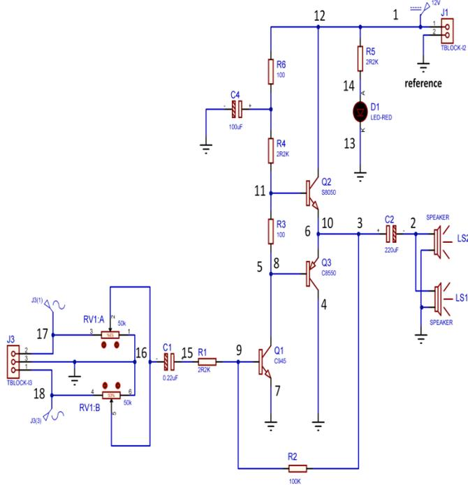
Figure 4. 2W Amplifier Schematic
