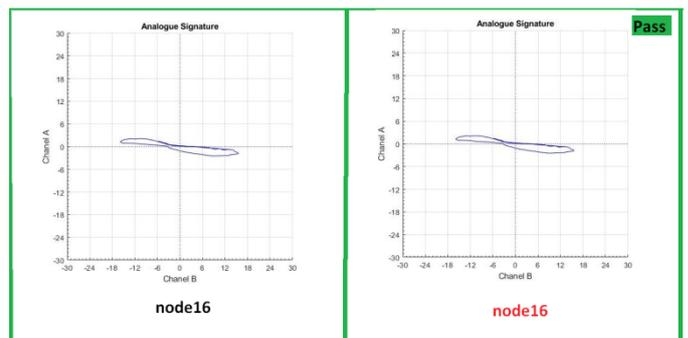
**Figure 11.** Analog signature on node16 of the cards after changing defective components
