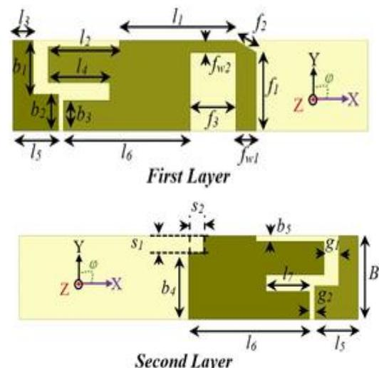
**Figure 1:** Schematic diagrams of the proposed antenna
