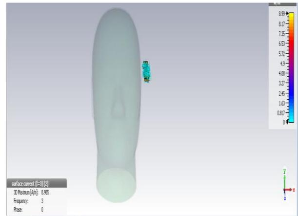
**Figure 13d:** Surface current at frequency 3 GHz
