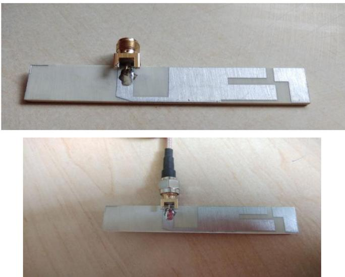
**Figure 6:** Prototype of the slot-loaded dipole antenna
