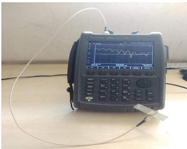
**Figure 7:** Slot-loaded dipole antenna connected with the VNA
