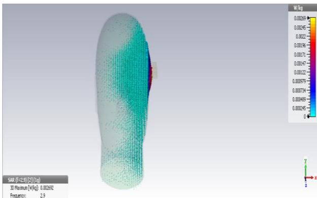
**Figure 13a:** SAR value at frequency 2.9 GHz
