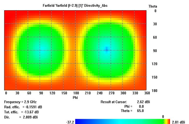
Figure 4: 2D far field radiation pattern at frequency 2.9 GHz
