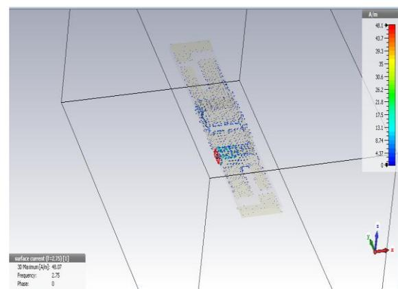
Figure 3: Current distribution of the proposed antenna
