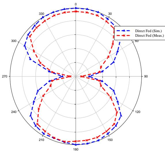
**Figure 11:** Radiation pattern of the antenna at frequency 2.9 GHz
