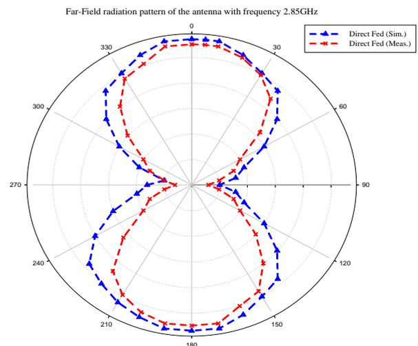
**Figure 10:** Radiation pattern of the antenna at frequency 2.85 GHz
