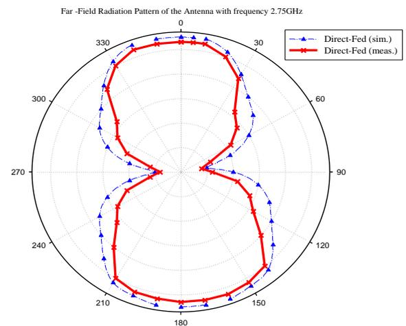
**Figure 9:** Radiation pattern of the antenna at frequency =2.75 GHz
