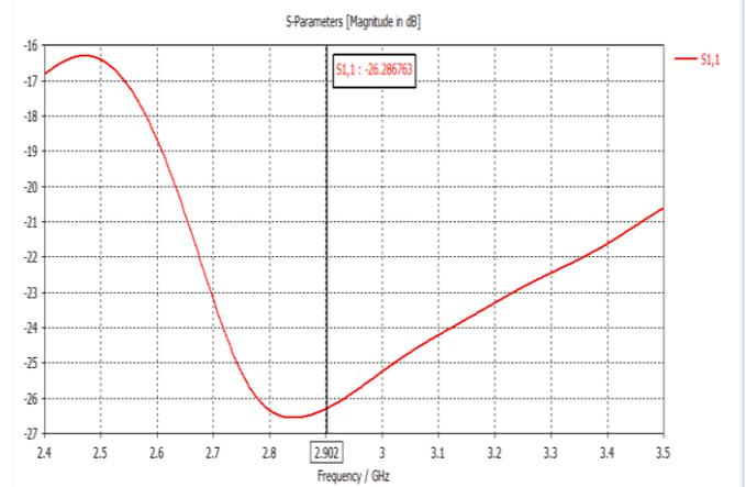
Figure 2: Reflection coefficient of slot-loaded dipole antenna
