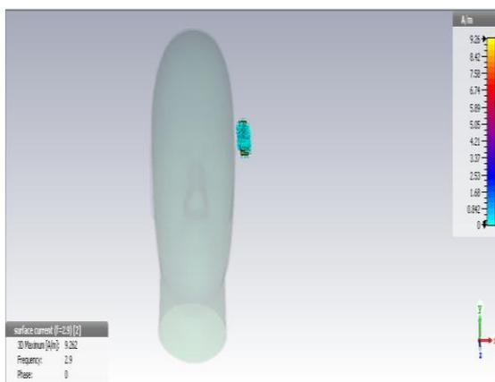
**Figure 13c:** Surface current at frequency 2.9 GHz
