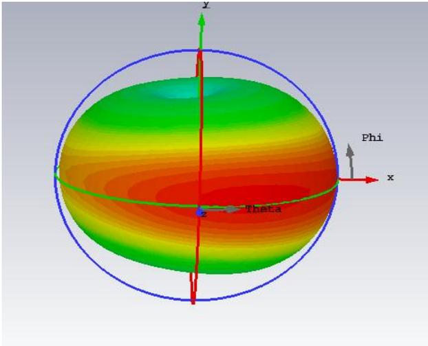
**Figure 5:** 3D view of far field radiation pattern at 2.9 GHz
