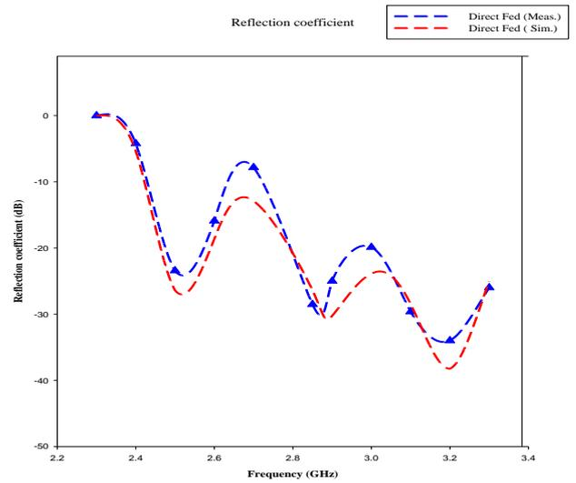
**Figure 8:** Comparison of reflection co-efficient of the antenna
