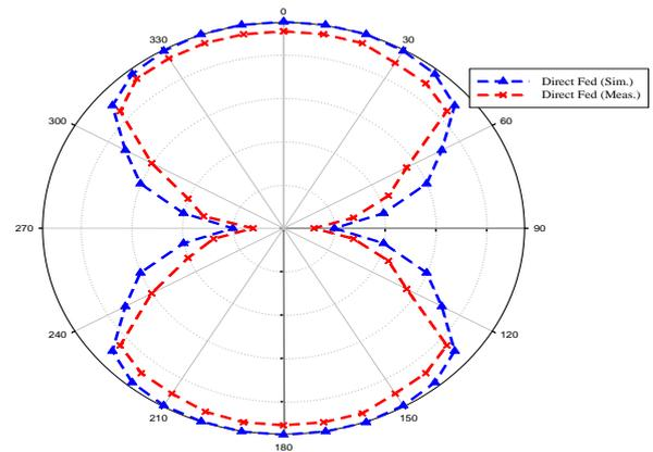
**Figure 12:** Radiation pattern of the antenna at frequency 3.08 GHz
