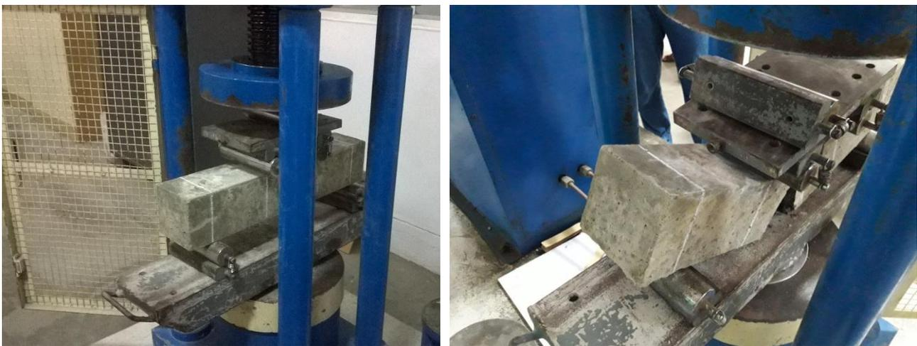
**Figure 8.** Flexural strength on Beam
