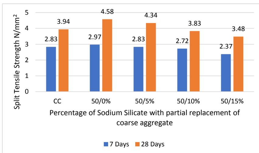
**Figure 6.** Split tensile strength for partial replacement of coarse aggregate with various percentage addition of sodium silicate
