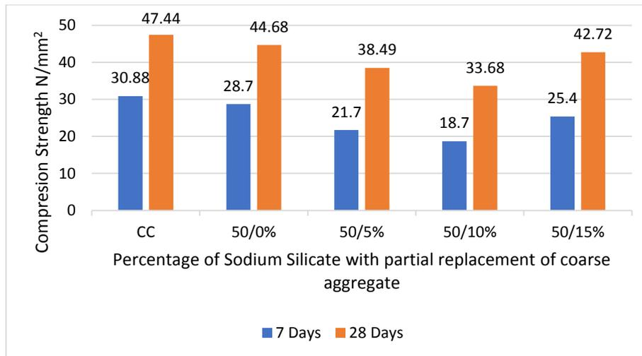
**Figure 3.** Compression strength for partial replacement of coarse aggregate with various percentage addition of sodium silicate
