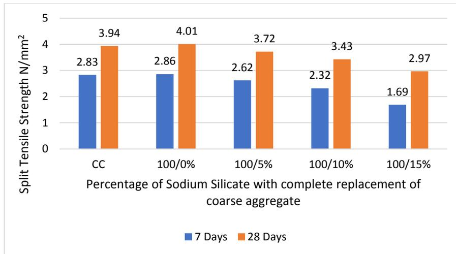
**Figure 7.** Split tensile strength for Complete replacement of coarse aggregate with various percentage addition of sodium silicate
