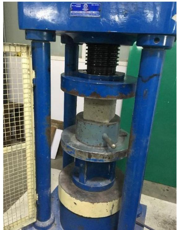
**Figure 2.** Compression strength on cube
