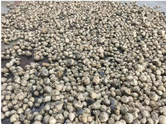
**Figure 1.** Fly ash aggregate
