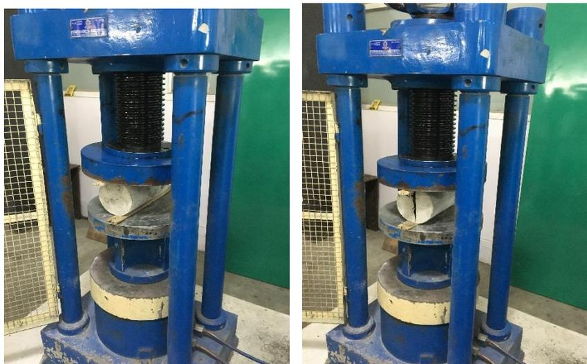
**Figure 5.** Split tensile strength on cylinder
