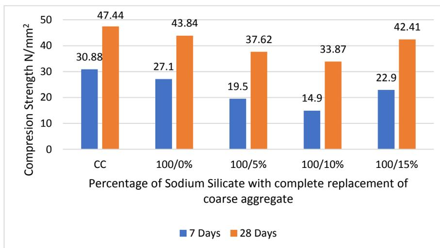
**Figure 4.** Compression strength for Complete replacement of coarse aggregate with various percentage addition of sodium silicate
