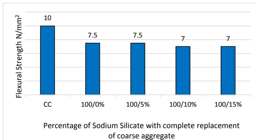
**Figure 10.** Flexural strength for Complete replacement of coarse aggregate with various percentage addition of sodium silicate
