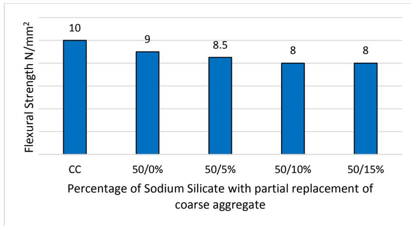
**Figure 9.** Flexural strength for partial replacement of coarse aggregate with various percentage addition of sodium silicate
