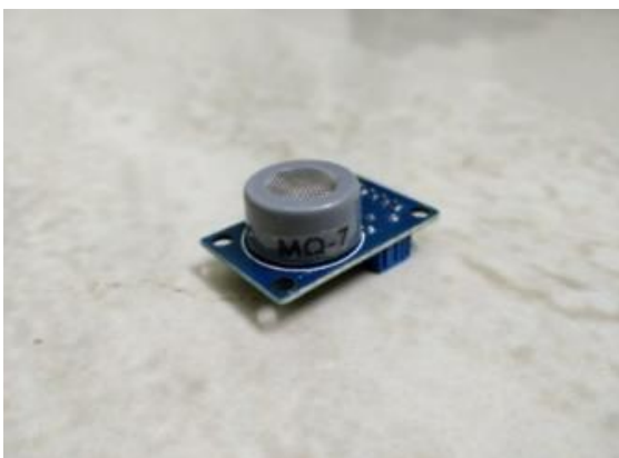
Figure 2. Sensing device for CO.
