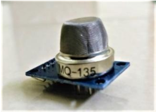
Figure 1. Sensing device for CO 2 .
