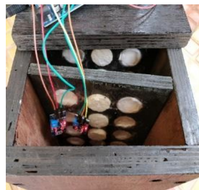
Figure 4. Programmed sensors arranged in the absorber.
