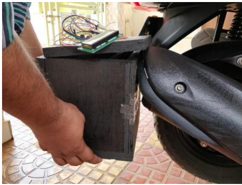
Figure 6. Exhaust of 4-stroke engine directed into absorber.
