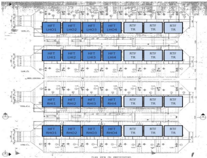
Figure 3: ESP power supply arrangement.
