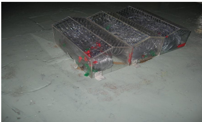
Figure 2.3 Model of three span pitched roof building
