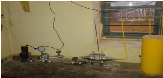
Figure 2. Image of actual setup of inducing hydrogen indicating safety measures
