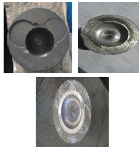
Figure 6. Images of hemi-spherical, toroidal and re-entrant toroidal pistons
