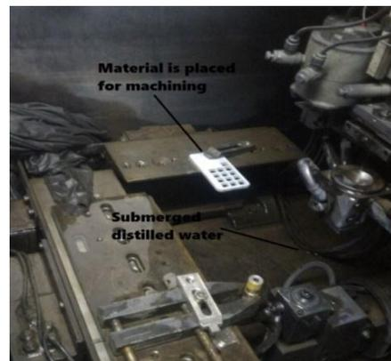
**Figure 3:** Photograph of the WEDM experimental setup
