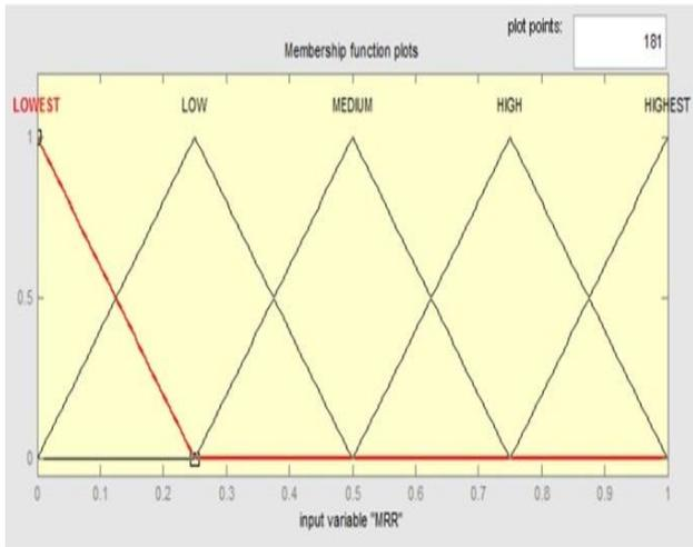
**Figure 4.** Membership functions for material removal rate and surface roughness
